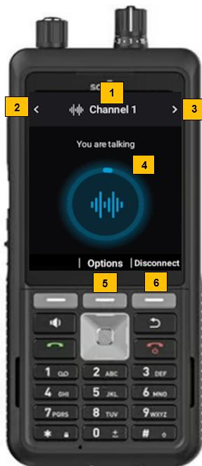
Joining a Channel screen
